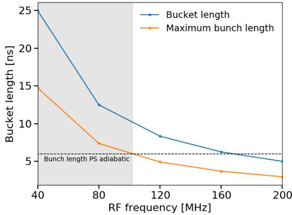
Figure 1: Bucket length and maximum bunch length for a filling factor  $q_p = 0.8$  and different RF frequencies of an SPS capture system.
