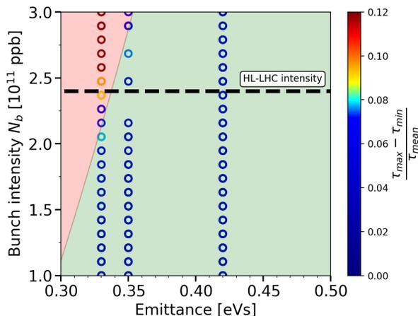
Figure 4: Stability threshold at the SPS flat bottom in a double 80 MHz and 200 MHz RF system in bunch-shortening mode with the full SPS impedance model after the LIU upgrades but without the impedance of the 80 MHz RF system. For every intensity,  $V_{80} = 1.1$  MV and  $V_{200} = 0.44$  MV. Colours represent the maximum relative amplitude of the bunch length oscillations during a 10 s flat bottom.
