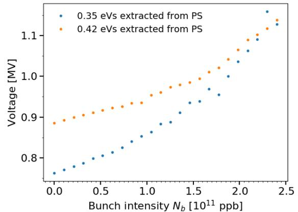
Figure 3: The matched 80 MHz capture voltage required in simulations in a double RF system to compensate for intensity effects and conserve the bunch length injected from the PS. The nominal and maximum emittances with  $q_p = 0.8$  are considered. The 200 MHz voltage in bunch-shortening mode is defined by Eq. (1).
