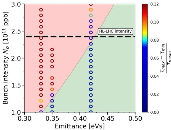
Figure 2: Stability threshold at the SPS flat bottom in a single 80 MHz RF system with  $V_{80} = 1.1$  MV and the SPS impedance model after the LIU upgrades but without the impedance of the 80 MHz RF system. Colours represent the maximum relative amplitude of the bunch length oscillations during a 10 s flat bottom.
