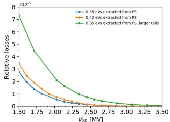
Figure 5: Relative losses in function of maximum  $V_{80}$  for 0.35 eVs and 0.42 eVs emittance beam. The intensity is fixed to  $N_b = 2.4 \times 10^{11}$  ppb and  $V_{80}$  at injection is 1.3 MV. The distribution with larger tails is binomial (see definition e.g. in Ref. [2]) with exponent of 5.
